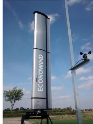
Figure 1.10: Measurements on the VentiFoil half scale model
