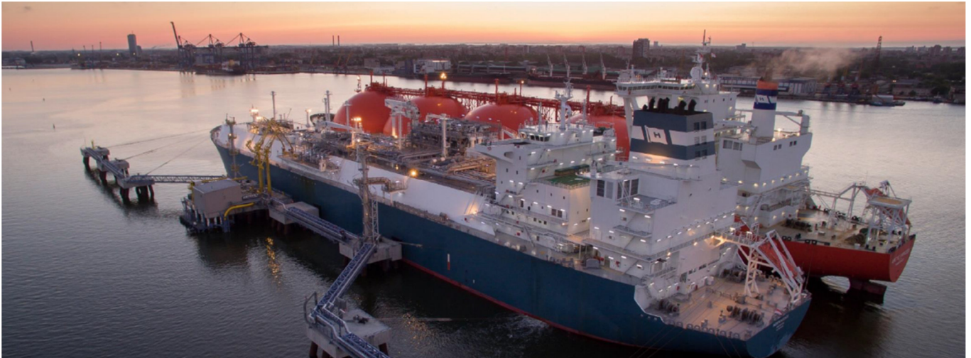
Figure 8 Typical FSRU berthing (170 000m 3 ) and LNGC offloading
